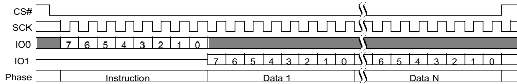
Figure 9-2 Read Identification (RDID 9Fh) Command Sequence
