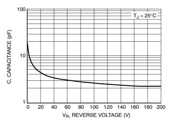
Figure 3. Typical Capacitance
