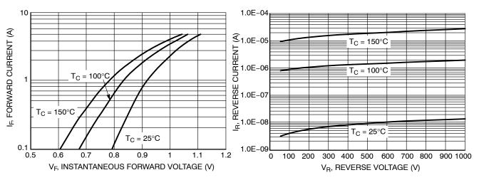
Figure 1. Typical Forward Voltage
