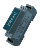
The KR4-I / U converter is used to convert a 4-20mA analog current signal into a 0-10V analog voltage signal. A 4-20mA current signal produced by any other electrical / electronic device can be provided for an analog input. The analog input can also be connected to a 2-wire passive transducer of any physical size (eg temperature, pressure) operating in the standard of 4 20mA
