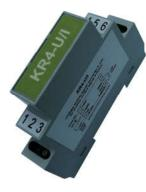
The KR4-U / I converter is used to convert the analog voltage signal 0-10V to a 4-20 mA analog current signal. The analog input can be supplied with a 0-10V voltage signal produced by any other electrical / electronic device. The signal from the analog output can control any electrical device with a 4-20 mA current input. For example, using the KR4-U / I converter, the voltage output of the PLC can be connected to an external device with a 4-20 mA current input.
