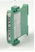
KSG I / U is primarily used to provide galvanic separation between two analogue signal circuits. In addition, it converts a 0-20mA or 4-20mA analog current signal into a 0-10V analog voltage signal.
