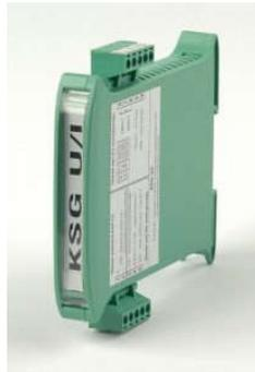
KSG U / I is primarily used to provide galvanic separation between two circuits of analog signals. In addition, it converts the analog 0-10V signal into a 0 / 4-20mA analog current signal.
