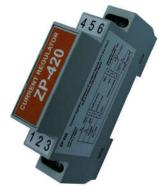
The ZP-420 current calculator is used to force a current of constant value of 4mA or 20mA, or an intermediate value determined by means of a resistor or a regulation potentiometer.
