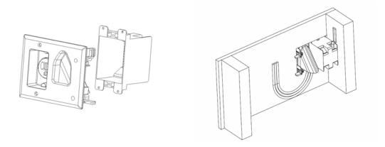
Once you have wired the receptacle, begin by inserting receptacle portion of the plate into the retrofit work box. Once the entire recessed plate is flush to the wall, using the two white screws supplied, screw the receptacle portion of the plate to the work box. **INSTRUCTIONS ARE CONTINUED ON THE BACK SIDE OF THIS PAGE**
