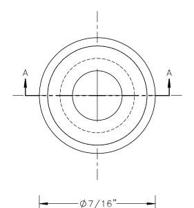
For use with panels of: Max Thickness = 0.093" Hole Dia. = 0.281"
