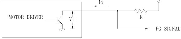
CAUTION: THE FG SINGAL LEAD WIRE MUST BE KEPT AWAY FROM "+" LEAD WIRE & "-" LEAD WIRE.
