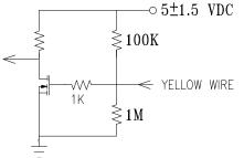
13-1. THE FAN SPEED WILL DEFAULT TO MAXIMUM WHEN THE SPEED CONTROLL INPUT IS LEFT UNCONNECTED.
