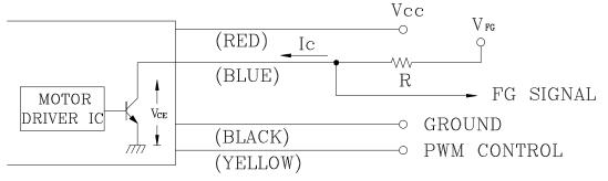
CAUTION: THE FG SINGAL LEAD WIRE MUST BE KEPT AWAY FROM "+" LEAD WIRE & "-" LEAD WIRE.
