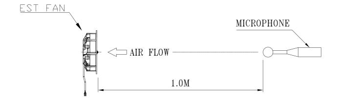
NOISE IS MEASURED AT RATED VOLTAGE IN FREE AIR IN SEMI-ANECHOIC CHAMBER WITH B & K SOUND LEVEL METER WITH MICROPHONE AT A DISTANCE OF 1.0M FROM THE FAN INTAKE.
