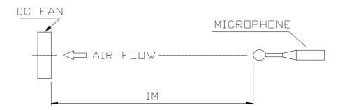
NOISE IS MEASURED AT RATED VOLTAGE IN FREE AIR IN SEMI-ANECHOIC CHAMBER WITH B & K SOUND LEVEL METER WITH MICROPHONE AT A DISTANCE OF 1M FROM THE FAN INTAKE.
