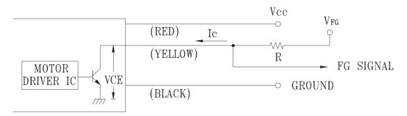
CAUTION: THE FG SIGNAL LEAD WIRE MUST BE KEPT AWAY FROM "+" LEAD WIRE & "-" LEAD WIRE.
