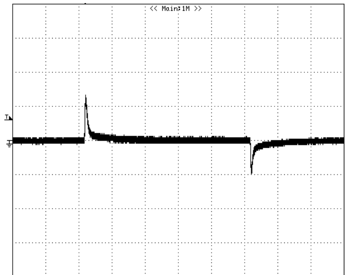
Figure 24: Typical transient response to step load change at 1A/\mu S from 100%~ 50%~100% of I_o , max at 12V_{in} , 0.59V_{out} ( C_{out} = 1\mu F + 47\mu F + 10\mu F ceramic) CH1 : VOUT, 0.1V/div, 200uS/div
