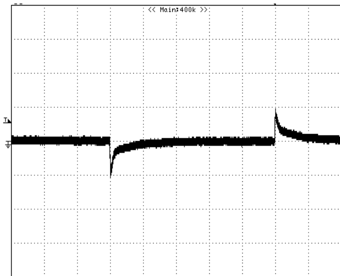
Figure 23: Typical transient response to step load change at 1A/\mu S from 100%~ 50%~100% of I_o , max at 12V_{in} , 1.2V_{out} ( C_{out} = 1\mu F + 47\mu F + 10\mu F ceramic) CH1 : VOUT, 50mV/div, 200uS/div
