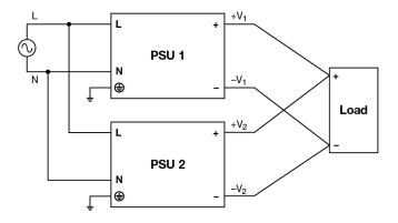
Fig. 5 Parallel Operation Connection Diagram
