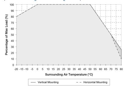
Fig. 1 De-rating for Vertical Mounting Orientation < 0°C de-rate power by 1% / °C,
