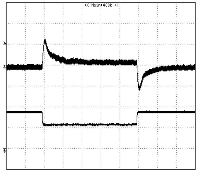
Figure 9: Output voltage response to step-change in load current (75%-50%-75% of I_o , max; di/dt = 2.5A/\mu s ). Load cap: 330\mu F , 35m\Omega ESR solid electrolytic capacitor and 1\mu F ceramic capacitor. Top Trace: V_{out} (100mV/div, 200us/div), Bottom Trace: I_{out} (5A/div). Scope measurement should be made using a BNC cable (length shorter than 20 inches). Position the load between 51 mm to 76 mm (2 inches to 3 inches) from the module
