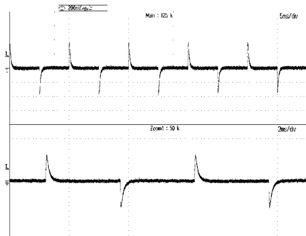
Figure 5: Output voltage response to step-change in load current (50%-75%-50% of full load; di/dt = 0.1A/\mu s ). Trace: Vout; 500mV/div; Time: 2ms/div
