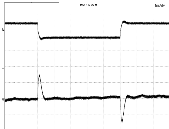
Figure 5: Output voltage response to step-change in load current (50%-75%-50% of full load; di/dt = 0.1A/\mu s ). Top Trace: Iout: 1A/div; Bottom Trace: Vout: 500mV/div
