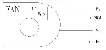
SIGNAL VOLTAGE RANGE:  $0 \sim (V_+ - 0.5)$  VDC
