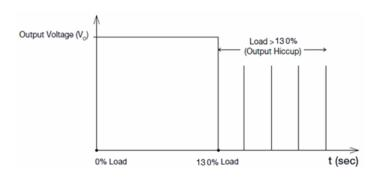
Additionally, if the  $I_0$  is <130% but >110% for a prolong period of time (depending on the load), the Over Temperature Protection (OTP) will be activated due to high temperature on critical components. The power supply will then go into hiccup mode until the fault is removed; and, the input voltage is removed, then reapplied.
