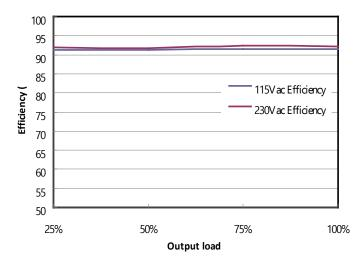
Fig.1 Efficiency versus output load
