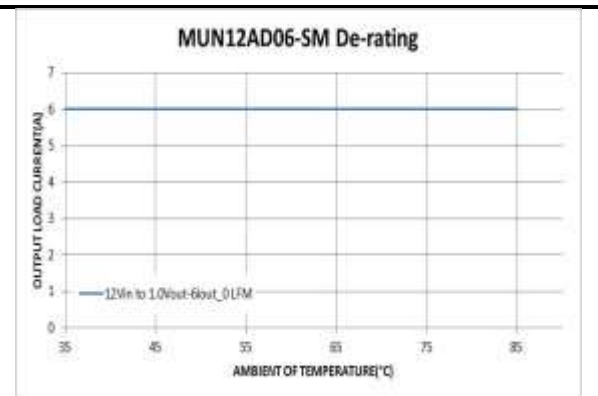
FIG.4 12VIN DE-RATING CURVE
