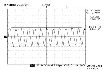
Figure 10: Output ripple & noise at 12 Vin, 1.5V/40A out
