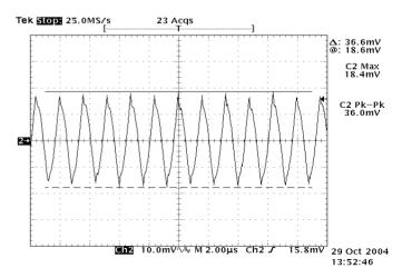
Figure 12: Output ripple & noise at 12 Vin, 2.5V/40A out
