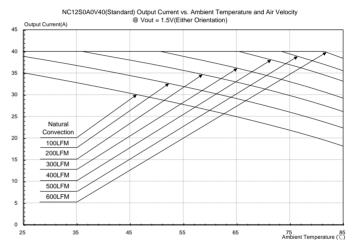
Figure 39: Output current vs. ambient temperature and air velocity @ Vout=1.5V(Either Orientation)
