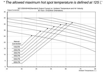
Figure 42: Output current vs. ambient temperature and air velocity@ Vout=5V(Either Orientation)
