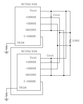
Figure 30: NC30/NC40 Current Sharing Diagram
