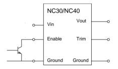
Figure 26: Enable Input drive circuit for NC series
