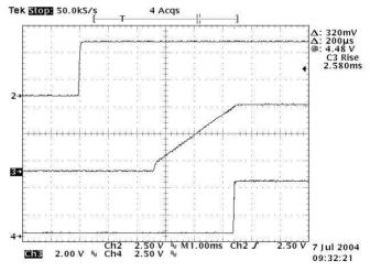
Figure 18: Turn on delay time Remote On/Off, 5V/40A out Ch2: ENABLE Ch3:Vout Ch4:PWRGD
