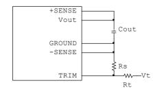
Figure 33: Output voltage trim with voltage source DS\_NC12S40A\_05282008
