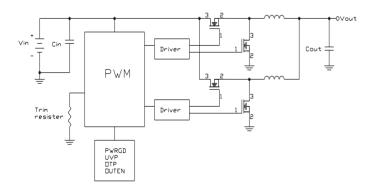
Figure 25: Block Diagram
