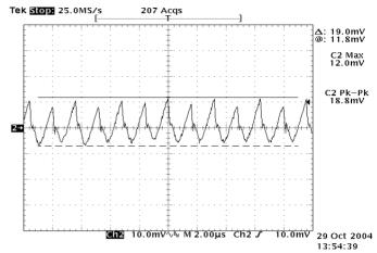
Figure 14: Output ripple & noise at 12Vin, 5V/40A out
