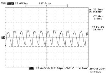
Figure 8: Output ripple & noise at 12 Vin, 0.9 V/40A out
