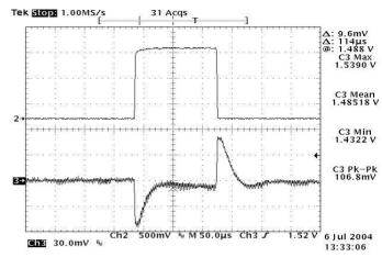
**Figure 20:** Typical transient response to step load change at  $10A/\mu$ S from 50% to 75% and 75% to 50% of lo, max at 12Vin, 1.5V out
