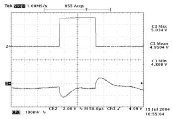
**Figure 24:** Typical transient response to step load change at  $10A/\mu$ S from 50% to 75% and 75% to 50% of lo, max at 12Vin, 5.0V out
