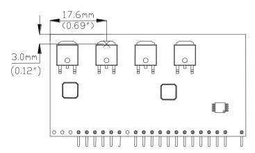
Figure 41: Temperature measurement location
