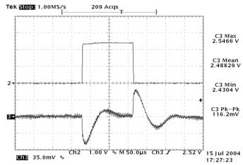
**Figure 22:** Typical transient response to step load change at  $10A/\mu$ S from 50% to 75% and 75% to 50% of lo, max at 12Vin, 2.5V out
