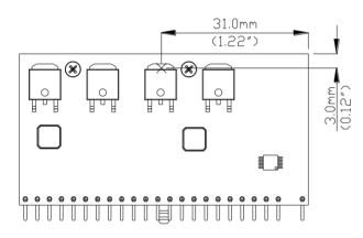
Figure 36: Temperature measurement location \* The allowed maximum hot spot temperature is defined at 125  $^\circ\!\!C$
