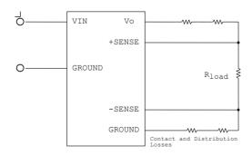
Figure 29: Circuit configuration for remote sense
