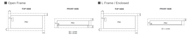
For safety reasons, please ensure the mounted device is kept at  $\geq 4$  mm safety distance at all sides from other components and equipments. Please insert an insulation sheet between the system and product, if the safety distance is less than 4mm.
