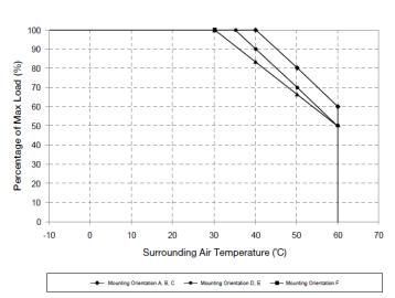
Fig.1.2 De-rating for Mounting Orientation A, B, C
