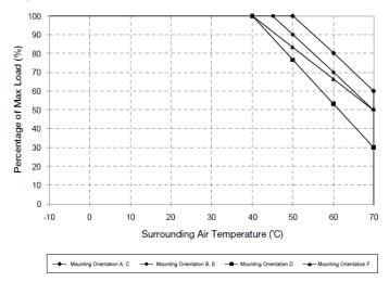
Fig.1.1 De-rating for Mounting Orientation A, C > 50°C de-rate power by 2% / °C
