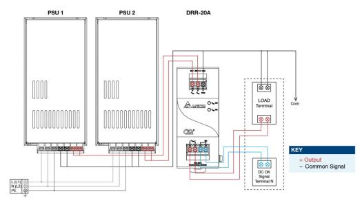
Fig. 5 Redundancy / Parallel Operation Connection Diagram
