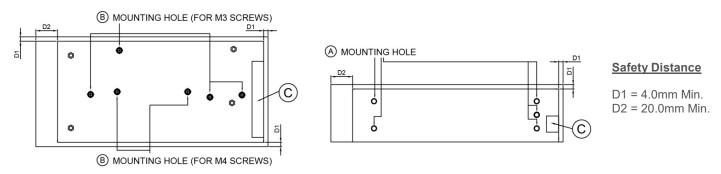
Fig. 3 Mounting Hole Locations and the Safety Distance
