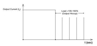
It is not recommended to prolong the duration of I<sub>O</sub> when it is <105% but >100%, since it may cause damage to the PSU.
