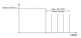
It is not recommended to prolong the duration of  $I_0$  when it is <105% but >100%, since it may cause damage to the PSU.
