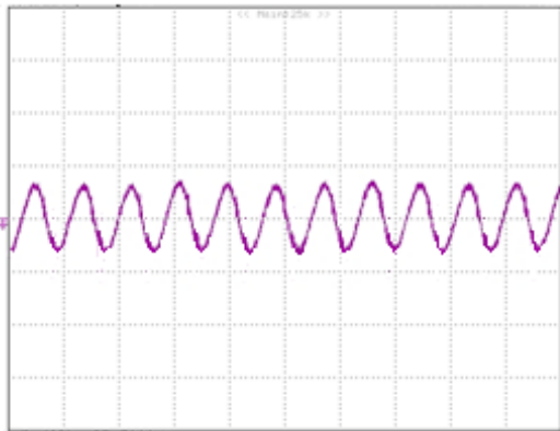
Figure 10: Input reflected ripple current, i_S , through a 12µH source inductor at nominal input voltage ( V_{in}=48V ) and rated load current (20 mA/div, 5us/div)
