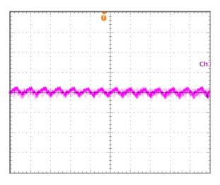
Input reflected ripple current, is, through a 12µH source inductor at nominal input voltage and rated load current (25 mA/div, 4us/div)
