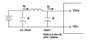
Test set-up diagram showing measurement points for Input Terminal Ripple Current and Input Reflected Ripple Current.
