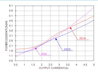
Power dissipation vs. load current at 25°C.
