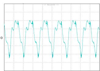
Output voltage ripple at nominal input voltage and max load current (20mV/div, 2us/div)
