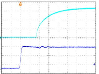
Turn-on transient at full load current (10ms/div). Top Trace: Vout; 1.5V/div; Bottom Trace: ON/OFF input: 2V/div.
