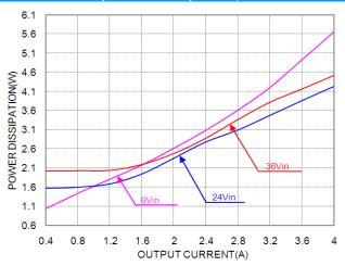
Power dissipation vs. load current at 25°C.
