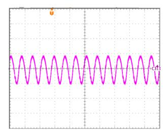
Input Terminal Ripple Current, ic, at full rated output current and nominal input voltage with  $12\mu H$  source impedance and  $100\mu F$  electrolytic capacitor (250 mA/div, 4us/div).
