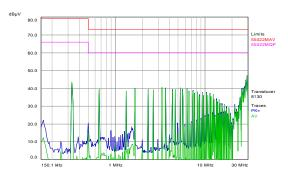
At T = +25°C, Typical input voltage and full load.
