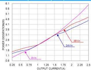
Power dissipation vs. load current at 25°C..
