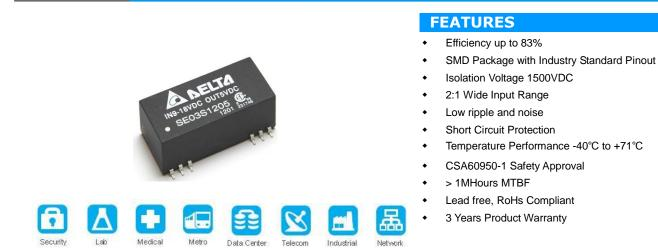
The SE03S/D series are miniature, SMD Package, isolated 3W DC/DC converters with 1,500VDC isolation. The SE03S/D series features fully regulated output and ultra wide 2:1 input voltage ranges. It offers short circuit protection and allows a wide operating temperature range of  $-40^{\circ}$ C to  $+71^{\circ}$ C. These isolated DC/DC converters are the latest offering from a world leader in power systems technology and manufacturing — Delta Electronics, Inc.
