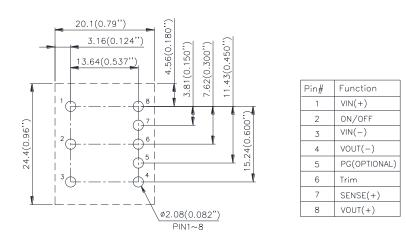
NOTES: DIMENSIONS ARE IN MILLIMETERS AND (INCHES) TOLERANCES: X.Xmm±0.5mm(X.XX in.±0.02 in.) X.XXmm±0.25mm(X.XXX in.±0.010 in.)
