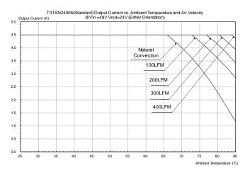
**Figure 30:** Output current vs. ambient temperature and air velocity @V<sub>in</sub>=48V, V<sub>out</sub>=24V (Either Orientation, Open Frame)
