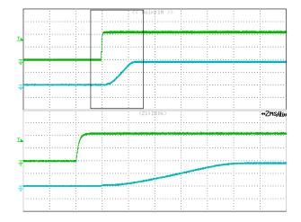
**Figure 12: Remote On/Off Start-up at open load** Time: 10ms/div. V<sub>remote On/Off signal</sub>(top trace): 2V/div; V<sub>out</sub> (bottom trace): 10V/div.
