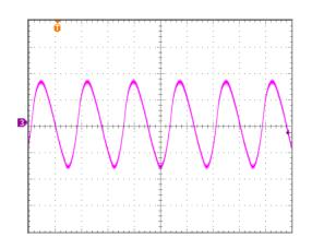
Figure 19: Input Terminal Ripple Current,  $i_c$ , at max output current, 48Vdc input voltage and 15Vdc output voltage with 12µH source impedance and 33µF electrolytic capacitor (500 mA/div, 2us/div).
