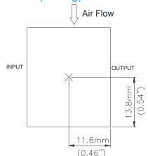
**Figure 31:** \* Hot spot temperature measured point. The allowed maximum hot spot temperature is defined at  $115^{\circ}$ C.
