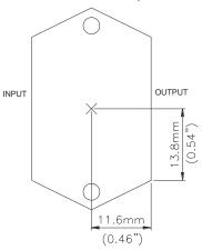
Figure 37: \* Hot spot on metal case temperature measured point. The allowed maximum hot spot temperature is defined at  $110^{\circ}$ C.
