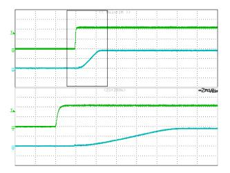
**Figure 13: Remote On/Off Start-up at full load** Time: 10ms/div. V<sub>remote On/Off signal</sub>(top trace): 2V/div;
