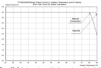
**Figure 33:** Output current vs. ambient temperature and air velocity @V<sub>in</sub>=48V, V<sub>out</sub>=18V (Either Orientation, Potting)
