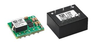
Non-isolated 1/32 Brick DC/DC Converter Input voltage: 9~53Vdc Single output: 5~30Vdc Output power: 100W
