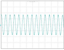
**Figure 22: Output Voltage Ripple and Noise** at 48Vdc input voltage, 24Vdc output voltage and max load current (20 mV/div, 5us/div)
