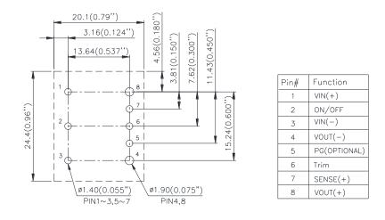
NOTES: DIMENSIONS ARE IN MILLIMETERS AND (INCHES) TOLERANCES: X.Xmm±0.5mm(X.XX in.±0.02 in.)
