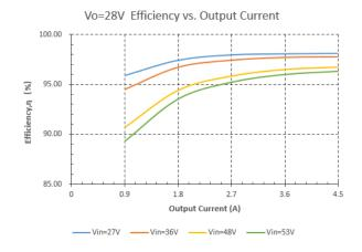
Figure 4: Efficiency vs. Output Current (Vo=28V)
