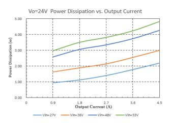
Figure 7: Power Dissipation vs. Output Current(Vo=24V)
