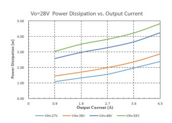
Figure 8: Power Dissipation vs. Output Current(Vo=28V)
