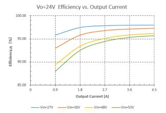
Figure 3: Efficiency vs. Output Current (Vo=24V)
