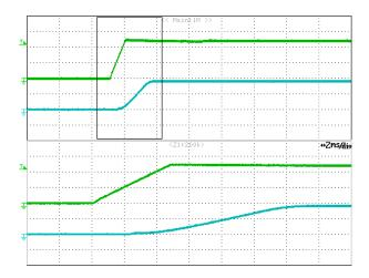
**Figure 14: Input Voltage Start-up at open load** Time: 10ms/div. V<sub>in</sub> (top trace): 20V/div; V<sub>out</sub> (bottom trace): 10V/div.
