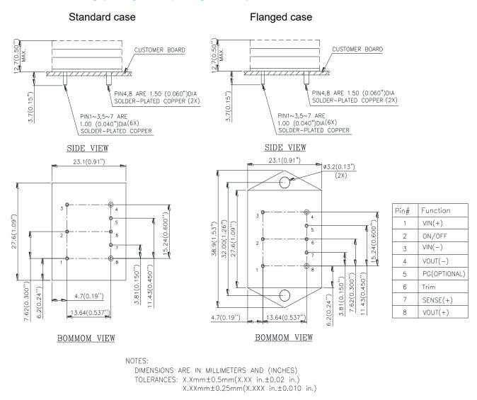
Note: All pins are copper alloy with matte Tin (Pb free) plated over Nickel under plating.
