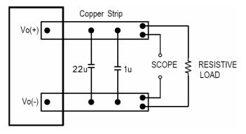
gure 21: Test Setup for Output Voltage Noise and Ripple
