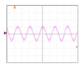
**Figure 20: Input Reflected Ripple Current**, is, through a 12µH source inductor at 48Vdc input voltage, 15Vdc output voltage and max load current (100mA/div, 2us/div).
