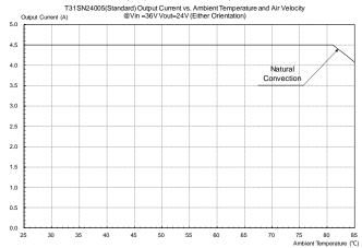
Figure 29: Output current vs. ambient temperature and air velocity @Vin=36V, Vout=24V (Either Orientation, Open Frame)
