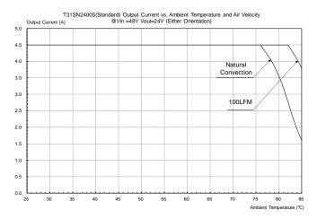
**Figure 35:** Output current vs. ambient temperature and air velocity @V<sub>in</sub>=48V, V<sub>out</sub>=24V (Either Orientation, Potting)
