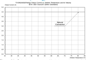
**Figure 34:** Output current vs. ambient temperature and air velocity @V<sub>in</sub>=36V, V<sub>out</sub>=24V (Either Orientation, Potting)
