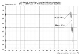
**Figure 38:** Output Current vs. Hot Spot on Metal Case Temperature @V<sub>in</sub>=24V&48V, V<sub>out</sub>=18V (Potting, Attach to Cold Plate)
