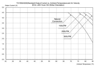
Figure 28: Output current vs. ambient temperature and air velocity  $@V_{in}=48V, V_{out}=18V$  (Either Orientation, Open Frame)
