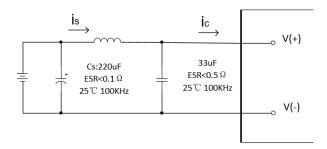
Figure 18: Test Setup Diagram for Input Ripple Current Note: Measured input reflected-ripple current with a simulated source Inductance ( $L_{TEST}$ ) of 12µH. Capacitor Cs offset possible battery impedance. Measure current as shown above.
