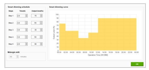
Note: When all steps are finished, the light level will remain in last level (level in step 5) for all three modes.
