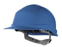
UV-resistant high density polyethylene (HDPE) or polypropylene (PP) safety helmet. Low density (LDPE) polyethylene cradle with 8 fixing points. Sweat band. Manual adjustment: head sizes 53/63 cm. Electrical Insulation up to 1 000 V.A.C. or 1 500 V.D.C. Standard holes for accessories. Anchorage for chin straps with 2 or 4 points.
