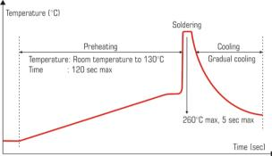
Fig.: Wave-soldering temperature-time profile to recommend
