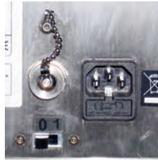
The interfacing socket, switch and power socket.
