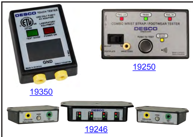
Figure 4. Wrist strap testers
