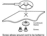
Screw allows ground cord to be bolted to mat to keep cord from disconnecting. NOTE: Use a punch or Philips screw driver to create a hole in the mat.
