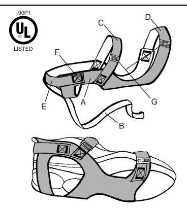
"For standing operations, personnel shall be grounded via a wrist strap system or by a flooring/footwear system. When a flooring-footwear system is used, one of the two following conditions shall be met:
