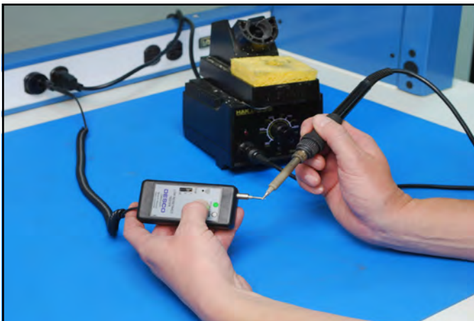
Figure 4. Testing a soldering iron with the 19245 tester
