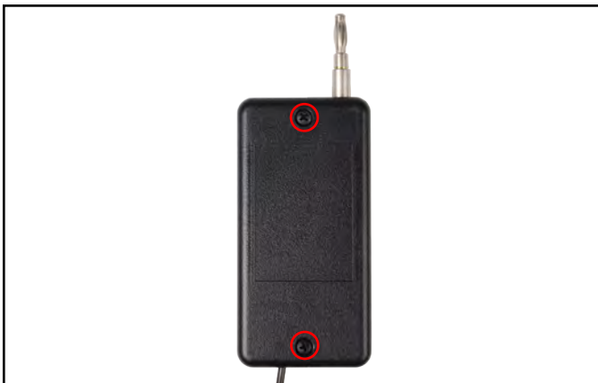
Figure 6. Locating the enclosure screws
