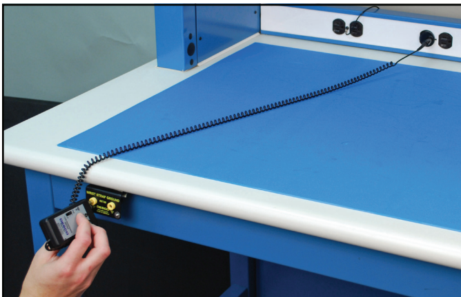
Figure 3. Testing ground points with the 19249 tester
