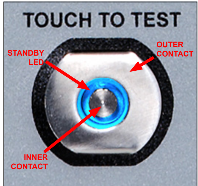
Figure 10. Steady-State Test Switch features and components
