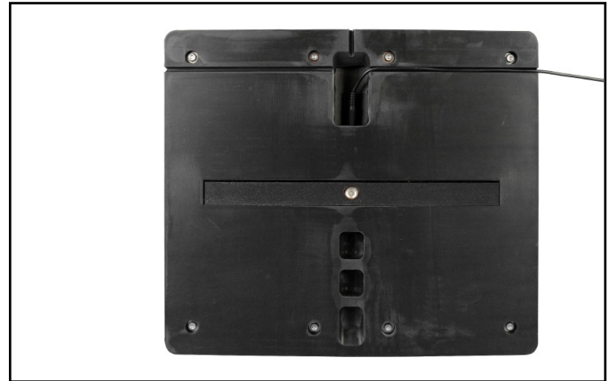
Figure 4. Routing the foot plate cord through the side
