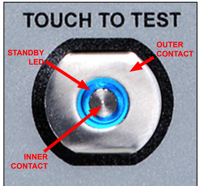
Figure 9. Steady-State Test Switch features and components
