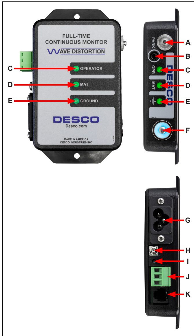
Figure 5. Full-Time Continuous Monitor features and components
