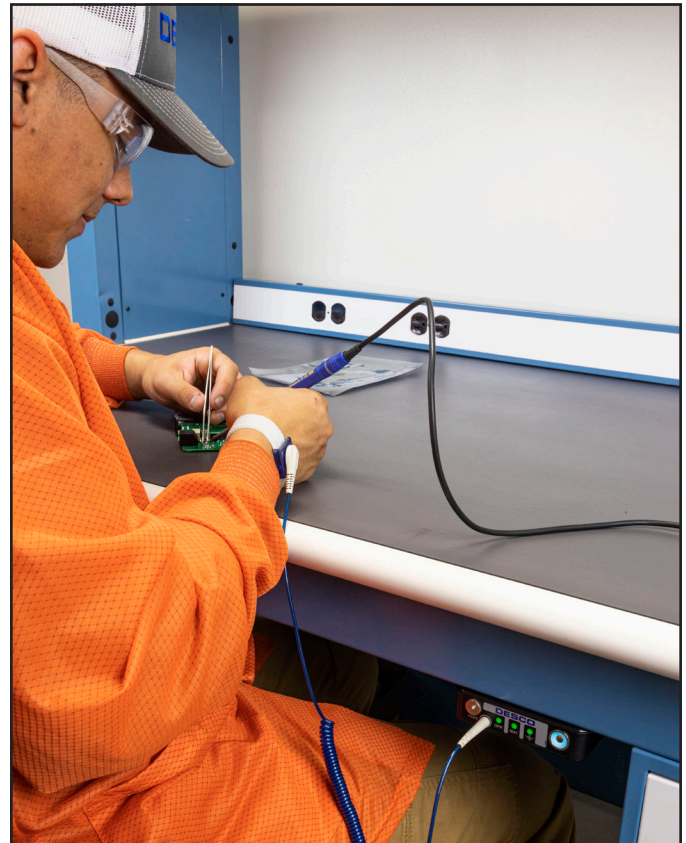
Figure 13. Using the Full-Time Continuous Monitor when mounted underneath a workbench tabletop
