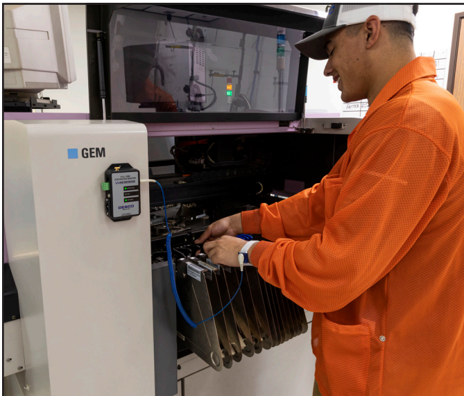
Figure 11. Using the Full-Time Continuous Monitor at a machine station
