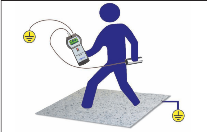
Figure 3. Setup of the Body Voltage Meter
