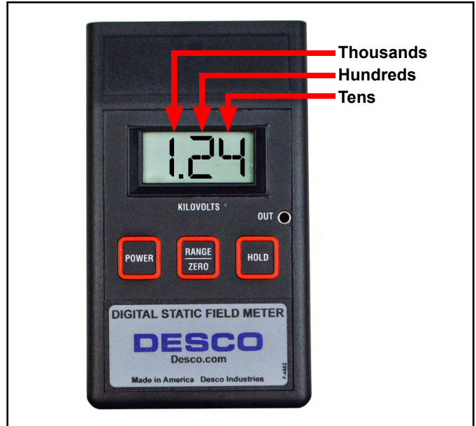
Figure 4. Reading the Digital Static Field Meter while in the \pm 20 kV range
