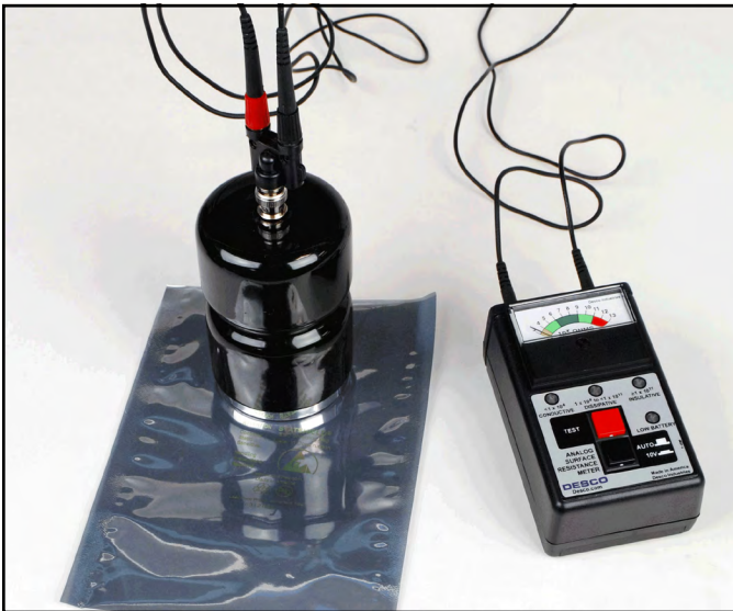
Figure 3. Using the Concentric Ring Probe with the Desco Analog Surface Resistance Meter
