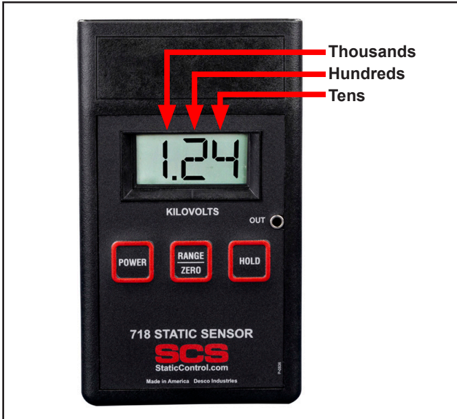
Figure 3. Reading the Static Sensor while in the \pm 20 kV range
