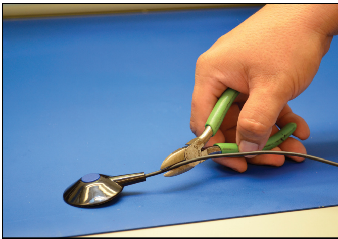
Figure 7. Cutting off table mat ground snap.
